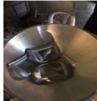
Gambar 4. Gambar Cacat Patah
