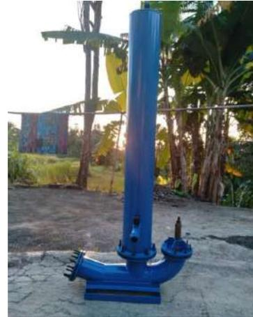
Gambar 4.1 Pompa Hidram
