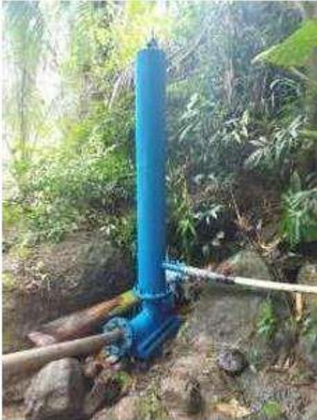
Gambar 4.1 Pompa Hidram
